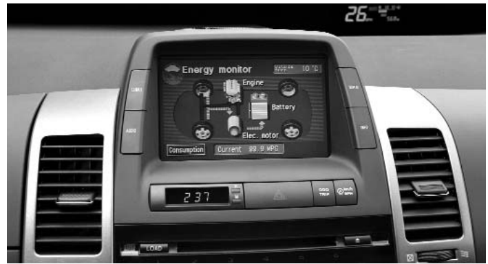
Energy monitor screen on the 2003 Toyota Prius. Although Toyota is hard to beat as an example of real excellence in engineering and build quality, the size and detail of this display hints that, for motorists, thinking about energy ought to be nearly as important as paying attention to the road.
